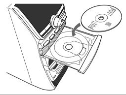
• When using an 8 cm disc, place it on the inner circle of the disc tray.
