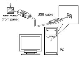
• Use "USB series A plug to B plug" cable when connecting.
